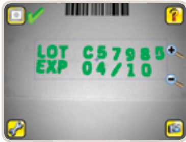
Match (Date/Lot Code Inspection)
