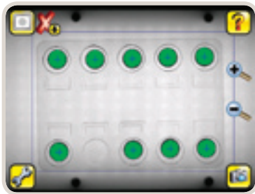
Area (Blister Pack Inspection)
